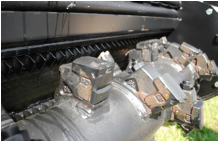
Single bolt carbide tooth retention
